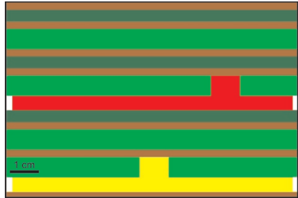
Fig. 5 Setup of the experiment. The yellow and red layers represent the buoyant PDMS, the light and dark green as well brown layers are the plasticine overburden.
